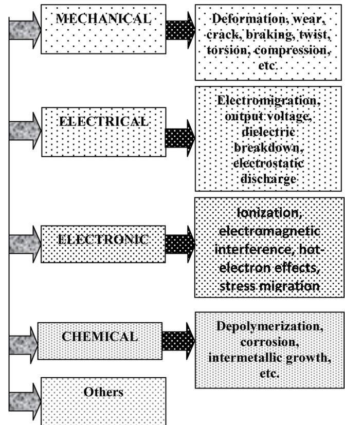
Figure 3. Types of physics-of-degradation mechanisms and their parameters.
